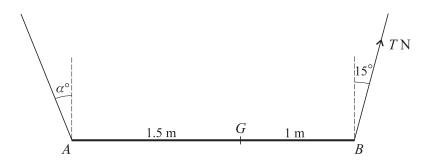
A non-uniform rod *AB* of length 2.5 m and mass 3 kg has its centre of mass at the point *G* of the rod, where AG = 1.5 m. The rod hangs horizontally, in equilibrium, from strings attached at *A* and *B*. The strings at *A* and *B* make angles with the vertical of  $\alpha^{\circ}$  and  $15^{\circ}$  respectively. The tension in the string at *B* is *T* N (see diagram). Find
